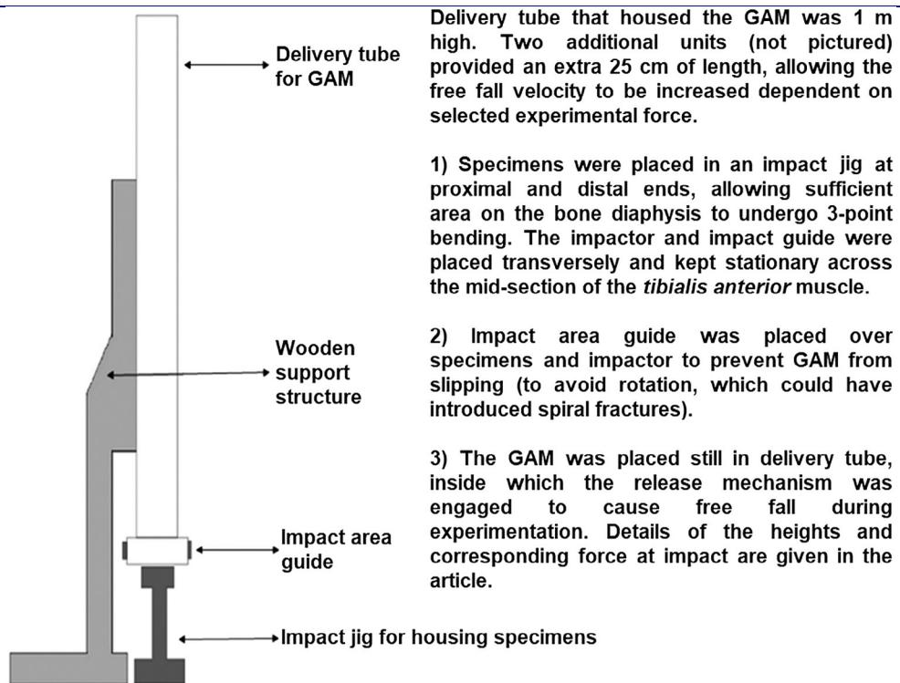
**Figure 2.** impact rig schematic.
